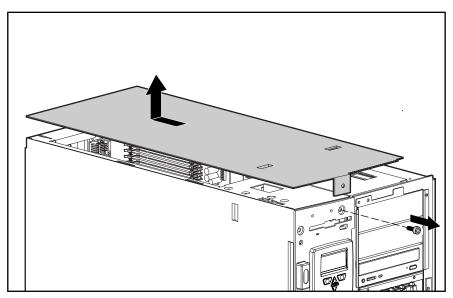
Figure 2-6. Removing the top access panel
